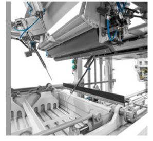
Precision filling system developed by Poyatos. Encoder controlled feeding box.
