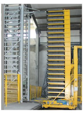
All-wheel drive automatic fingercar for increased operating speed.
