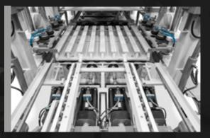
2 independent vibration tables for better filling compensation. Greased in permanent oil bath (minimum maintenance).
