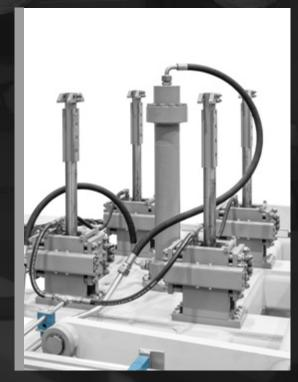
Brakes to block the tamper during demoulding.
