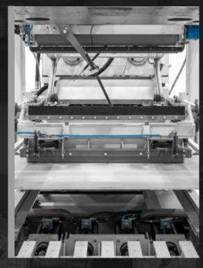
Elevation of the box frame in its reverse gear to manufacture large slabs.
