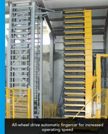
All-wheel drive automatic fingercar for increased operating speed
