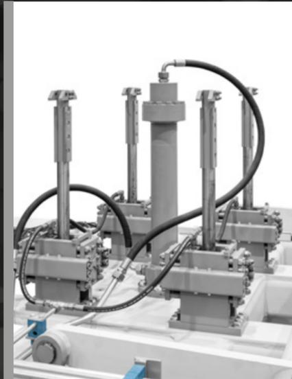
Brakes to block the tamper during demoulding.
